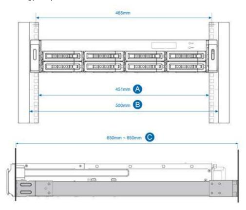
2. The rack kits for the VS-8100U-RP Pro rack mount series are only compatible with square-hole server racks.
